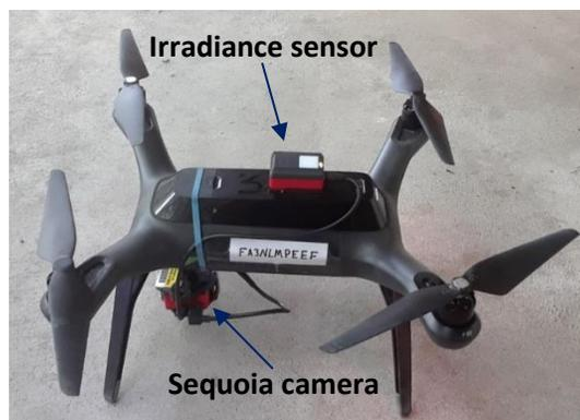
**Figure 1.** A Solo UAV and a Sequoia camera used for collecting aerial images of the field.
